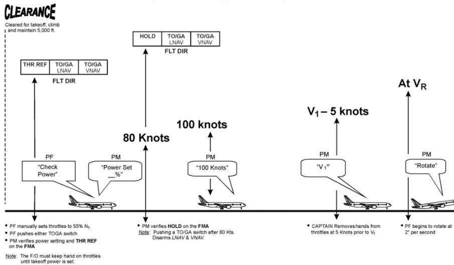
**Normal Takeoff Profile (Modified ICAO A) (LNAV & VNAV) Initial Climb ( $V_2 + 15$  Knots) And Acceleration**
