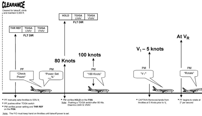
**Alternate Takeoff Profile (Modified ICAO B) (LNAV & VNAV) Initial Climb ( $V_2 + 15$  Knots) And Acceleration**
